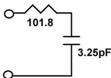
**Screen 4, Parallel Impedance:** Displays the resistive and reactive components as two parallel elements. Also displays true reactance plus a finite inductive or capacitive value.
