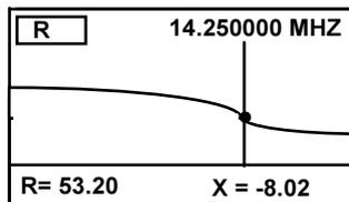
**Reactance Screen (+X or -X):** The *Reactance* plot tracks both reactive value and displays sign to accurately identify if the load is capacitive or inductive. The resistive component is also shown.
